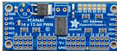
Figure 113: Adafruit PCA9685 I 2 C interface PWM Servo Controller
