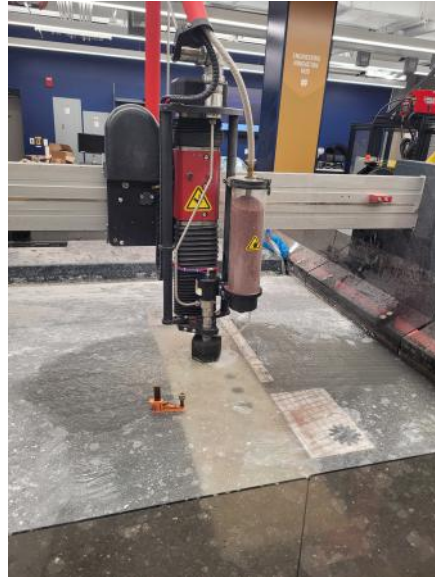
Figure 25: Water Jet Cutting Submerged G10 Fiberglass Sheet
