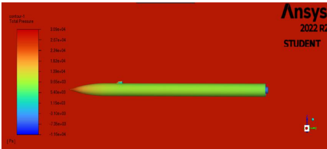
Figure 84: 2D CFD Model of the Pressure Over the Surface
