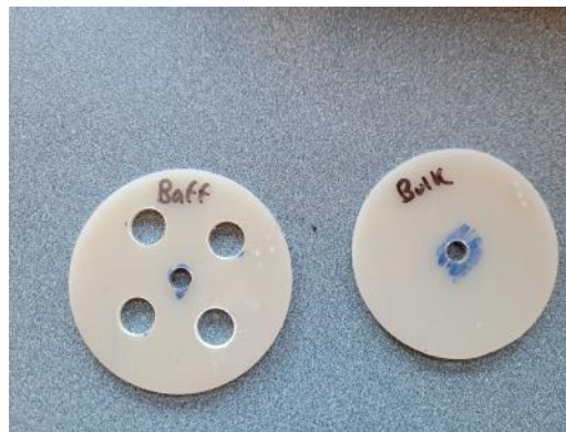
Figure 26: Baffle and bulkhead
