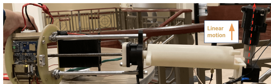
Figure 62: TROI Step 3: Telescoping Camera Arm Deployment
