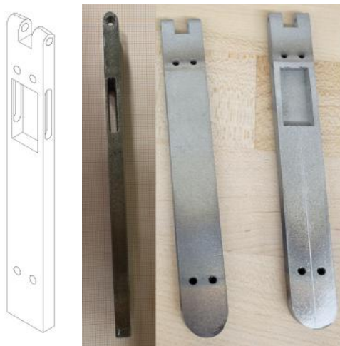
Figure 80: CAD Drawing (left) and as constructed (right) flap lever arms
