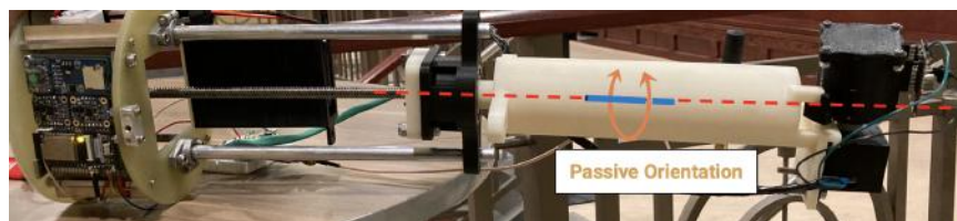
Figure 61: TROI Step 2: Bearing Rotation
