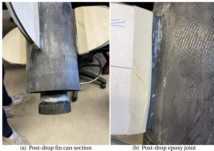
Figure 122: Results of fin can drop test
