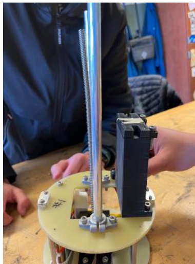
Figure 75: Lead Screw Damage after VDF Attempt
