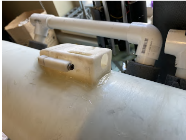
Figure 22: Camera Shroud Epoxied to Payload Tube
