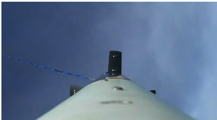
Figure 97: In-flight ACS Drag Flap Deployment
