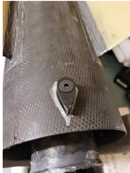
Figure 21: Rail Buttons Epoxied to Fin Can
