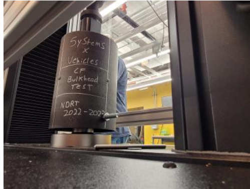
Figure 124: Bulkhead static loading test setup
