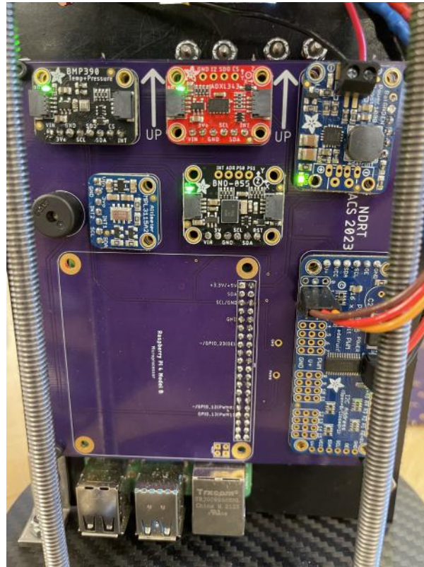
Figure 86: Battery-powered PCB with mounted electronics (armed)
