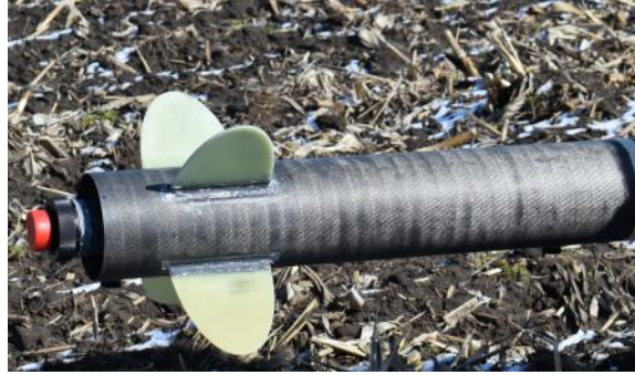
Figure 30: Constructed Fin Can
