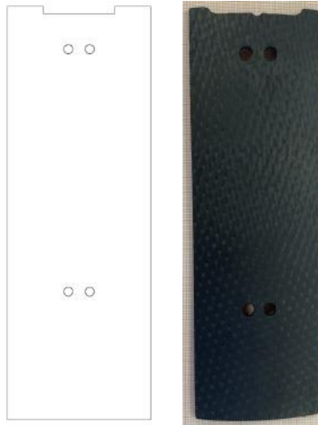
Figure 81: CAD Drawing (left) and as constructed (right) drag flap
