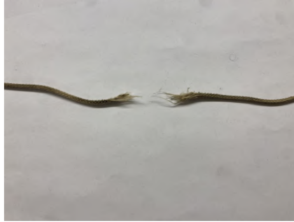
Figure 93: Broken Shock Cord
